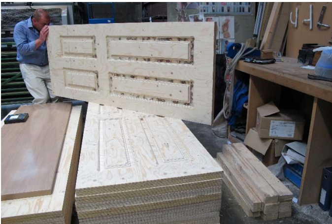
Figure 42: Dimensionally precise and strong Kerto-Q panels for door frameworks.
