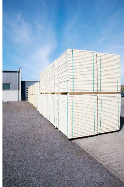
Figure 41: Strong, long and light Kerto-Q panels coated for use as base plates in the concrete product industry.
